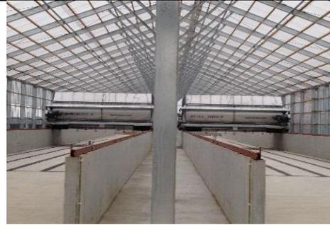
Fermented chicken manure processing system developed by Sunki Biotech.
